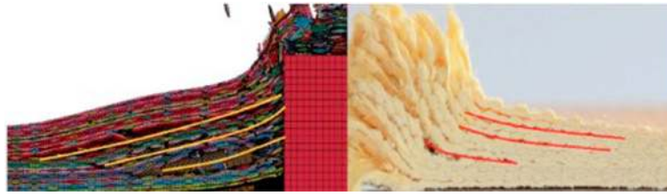
Fig. 18 Comparison of experimental tests with damage morphology obtained with meso-heterogeneous model (Bresciani et al. 2016)
