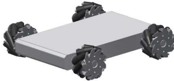
Fig.2. Virtual model of a WMR with mecanum wheels.
