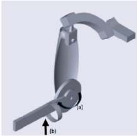
Fig. 13. Exoskeleton: a) exoskeleton movement and b) external disturbance
