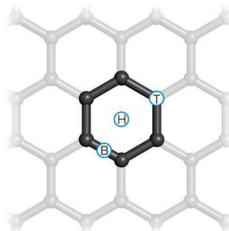
Fig. 9 On bond (B), top (T), and hollow (H) adsorption sites on graphene.
