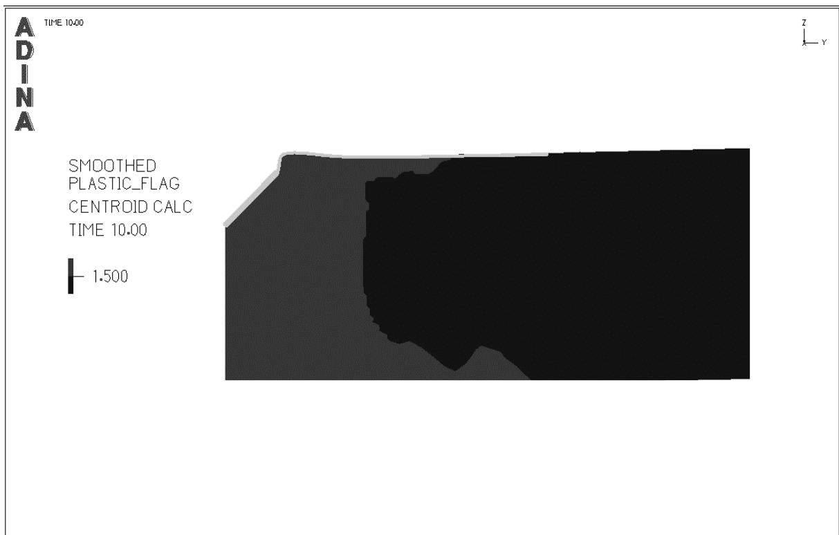
Fig. 11. Area of the crack formation for the sharp indenter
