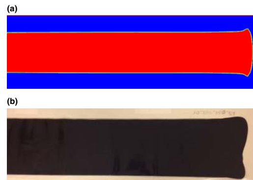
Fig. 10. Increased value of side flow in the beginning of the tape for the highest value of initial slurry height (20.8 mm) for (a) numerical prediction and (b) experimental tape casting.
