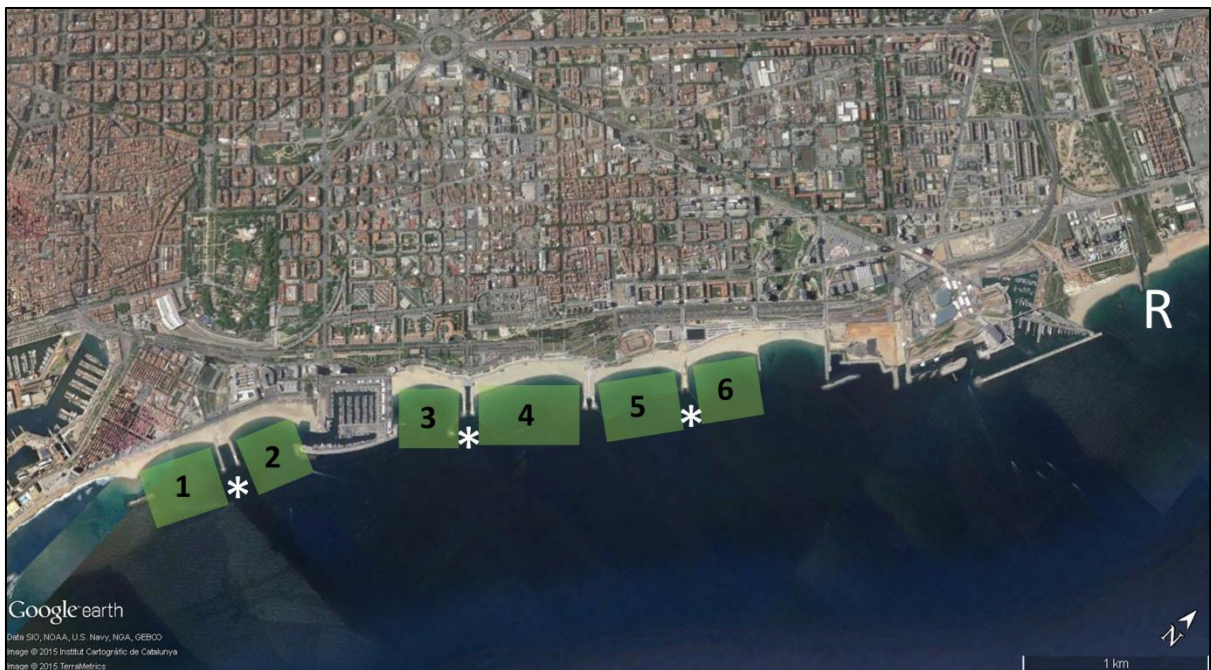
Fig. 8: Map of the Barcelona beaches affected by combined sewer overflows and by the River Besòs. The beaches are (1) Andrea Doria; (2) Hospital del Mar; (3) Nova Icària; (4) Bogatell; (5) Mar Bella; and (6) Nova Mar Bella. The map also indicates the position of the CSO outlets (*) and the River Besòs (R). (Google Earth, Cartographic Institute of Catalonia)
