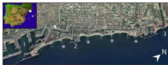
Fig. 1. Coastline of Barcelona, indicating beaches, industrial harbors (1), recreational harbors (2), combined sewer overflow outlets (*), and the mouth of the River Besòs (3). (Data source: Cartographic Institute of Catalonia)
