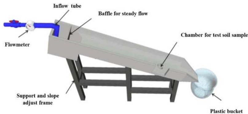
Figure 3. Schematic representation of the hydraulic flume.
