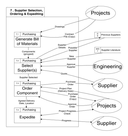
Figure 4 Data Flow Diagram - Supplier Selection, Ordering and Expediting
