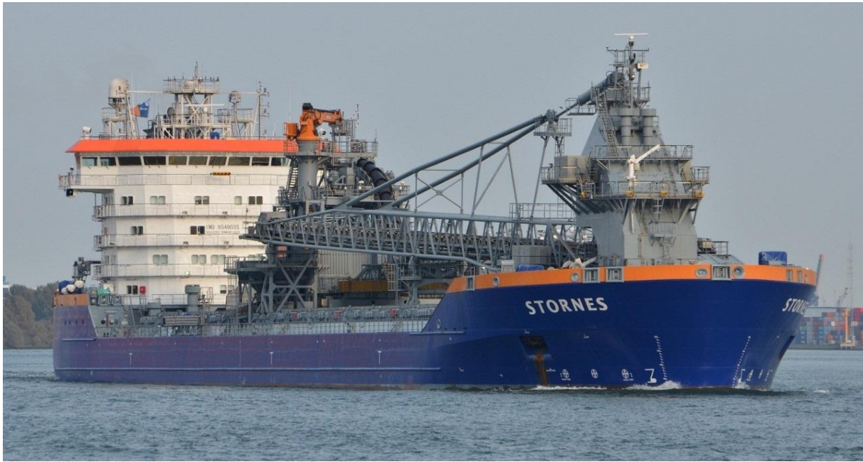
Figure 15.3: Flexible fallpipe vessel Stornes
