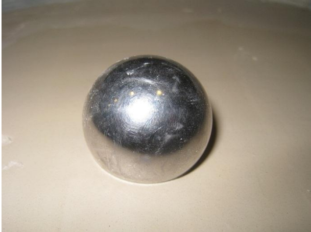
Figure 15.30: Particle penetration \Delta = 0.008 m ( D_s = 30 mm, \rho_s = 7821 kg/m 3 , v_{imp} = 2.0 m/s)
