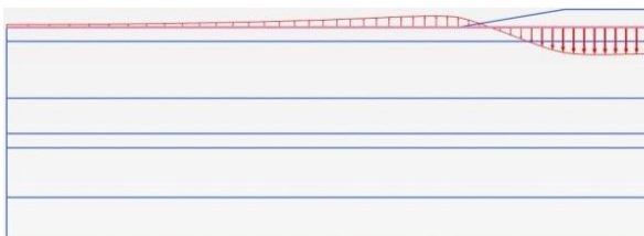
Figure 15.65: Vertical deformation over the length of the berm
