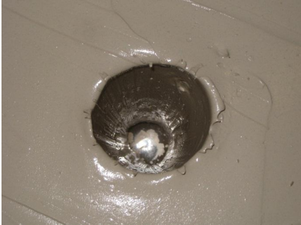
Figure 15.21: Particle penetration \Delta = 0.069 m ( D_s = 30 mm, \rho_s = 7821 kg/m 3 , v_{imp} = 3.0 m/s)
