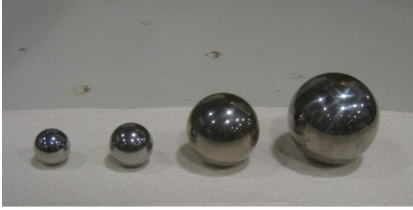
Figure 15.18: Steel bearings in different sizes ranging from 15 mm to 38 mm diameter
