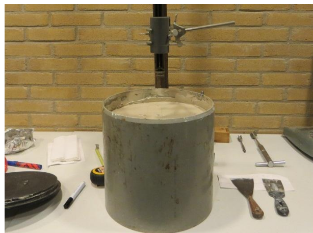
Figure 15.17: Test setup single stone fall experiment ( v_{imp} = 2 \text{ m/s} )
