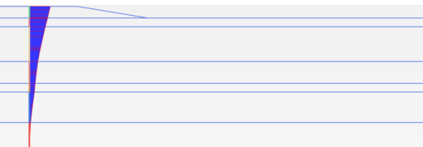
Figure 15.66: Vertical deformations over the depth seabed berm
