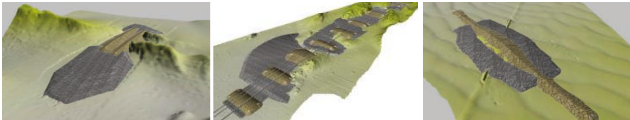
(a) The basic design of supports (brown) (b) Free span mitigation supports (brown) including counter fills (grey) (c) Support for a pipeline crossing (brown) and counter fill (grey)
