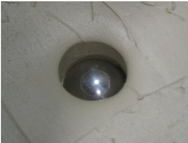
Figure 15.27: Particle penetration \Delta = 0.040 m ( D_s = 30 mm, \rho_s = 7821 kg/m 3 , v_{imp} = 4.0 m/s)
