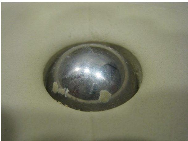
Figure 15.34: Particle penetration \Delta = 0.033 m ( D_s = 30 mm, \rho_s = 7821 kg/m 3 , v_{imp} = 6.0 m/s)
