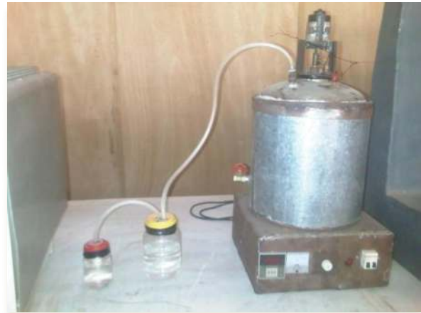
Fig. 1. Experimental set up for biogas production
