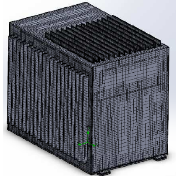
Fig.7 Three dimensional meshed model of space optimized EU
