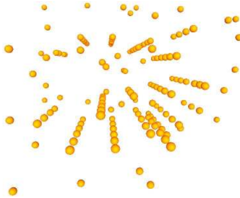
Figure 1.1: Example of a dataset in geology, where samples were collected by drilling a hole in the ground. Each sample has a location in 3D space ( x - y - z coordinates) and one or more attributes attached to it.
