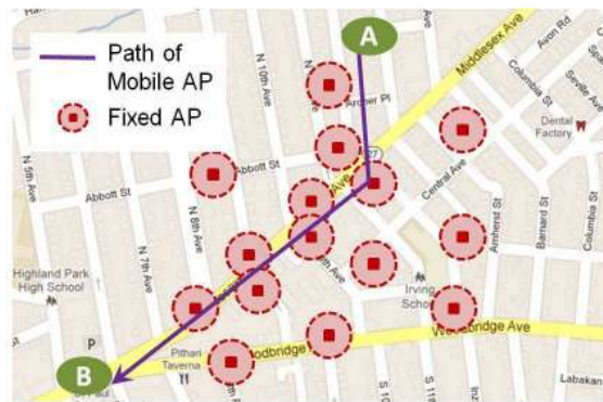
(a) A user traveling with a mobile WLAN from point A to B can be in range of a varying number of fixed WLANs
