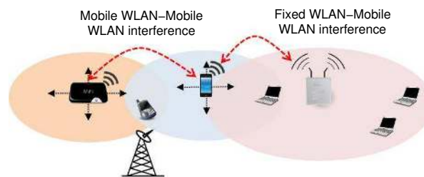
(b) Intra-mobile WLAN and mobile WLAN-fixed WLAN interference.
