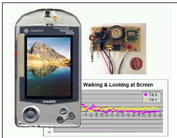
Figure 7. Sensing PDA, outfitted with multiple perceptual sensors, including proximity, motion, and touch sensors. In the background, accelerometer signals are displayed showing the motion fingerprint of a user walking while looking at the device.
