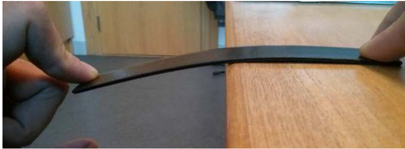
FIGURE 2.2. A deformed ruler caused by forces applied at both ends of the ruler as well as at the center of the ruler (reactive force form the table).
