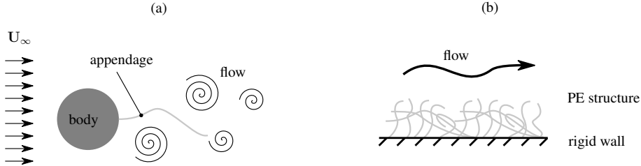
FIGURE 1.5. A sketch of the problems investigated in this work. In frame (a), a bluff body with an appendage is exposed to uniform free stream U_\infty . In frame (b), a poroelastic (PE) structure is added on top of a rigid wall, which is exposed to a free fluid flow above it.
