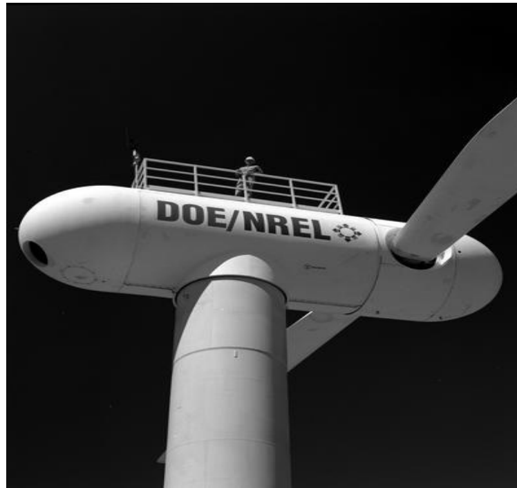
Figure 2-6. The Controls Advanced Research Turbine (CART)
