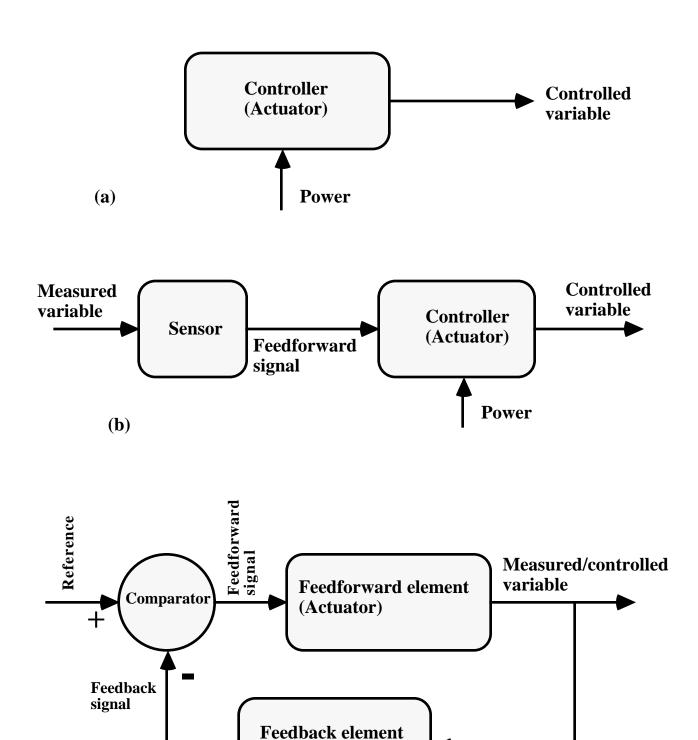
Figure 2. Different Control Loops for Active Flow Control.
