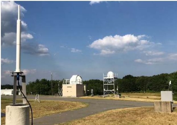
Fig. 3 DORIS beacon at GGAO with the NGSLR prototype system in the background. The SLR aircraft avoidance radar is located on the tower to the right of the NGSLR shelter
