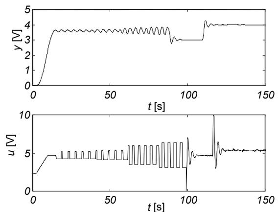
Fig. 6. Autotuning experiment on the process simulator.
