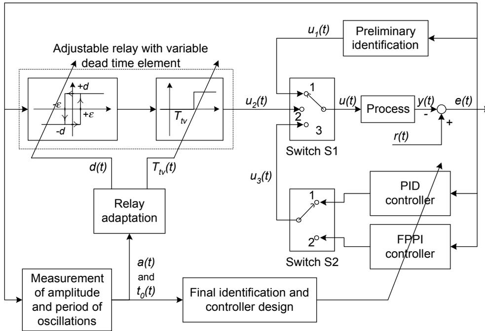
Fig. 2. Structure of the modified autotuning PID controller.
