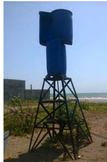
Figure 4. Real construction of the double Savonius
