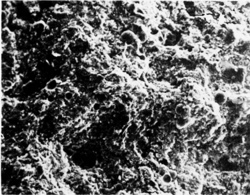
Figure 15. Micrograph 072380-12, X 190. Fracture surface of Mixture M-8-A at 7-day age. Surface shows more void space than Figure 16.
