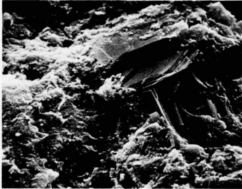
Figure 21. Micrograph 110780-10, X 2000. Fracture surface of Mixture M-9-F at 90-days age. Dense structure showing massive calcium hydroxide (center) surrounded by CSH. The number of elongated voids seen at the 3-day age (Figure 10) has decreased with time.
