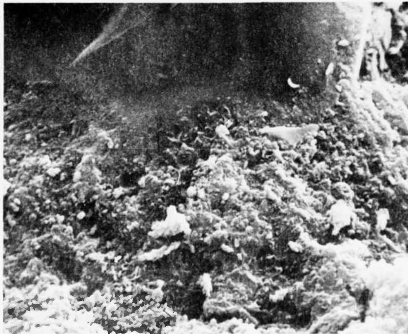
Figure 13. Micrograph 081380-6, X 2000. Fracture surface of Mixture M-8-A at 28-days age. The ash sphere in the center is believed to represent removal of glass by hydration leaving resistant crystalline phases such as quartz and mullite behind.
