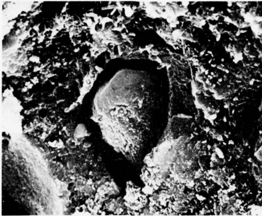
Figure 1. Micrograph 080280-23, X 4900. Fracture surface of Mixture M-8-D at 7-day age. Partially hydrated cement grain in center (Hadley grain, Reference 5).
