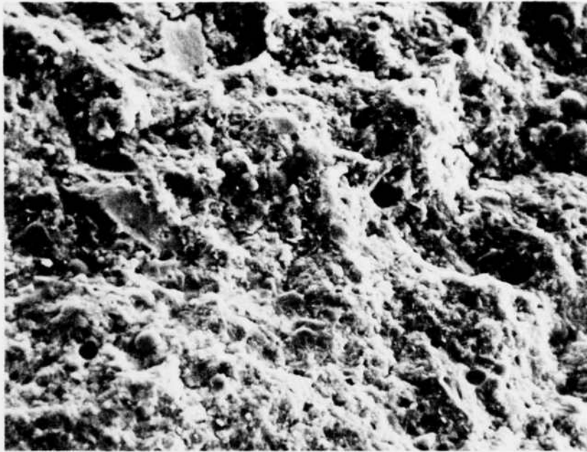
Figure 17. Micrograph 081280-17, X 200. Fracture surface of Mixture M-9-F at 7-day age showing residual unhydrated cement, fly ash spheres, hydration product, and void space.
