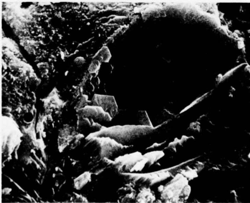
Figure 8. Micrograph 082680-47, X 2200. Fracture surface of Mixture M-9-C at 28-days age. Calcium hydroxide crystals in void surrounded by CSH and calcium hydroxide.
