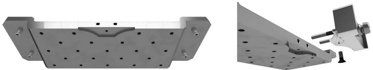
Fig. 6 Detailed view of pallet modifications
