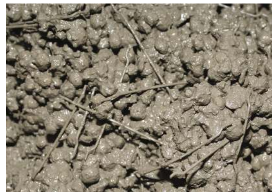
Fig. 1. Concrete mixture before compaction (IIS3)
