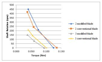
Figure 7. Graph of the relationship between shaft rotation and torque with turbine blade variations
