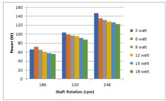
Figure 9. Graph of the relationship of electric power to shaft speed with variations in load on a conventional 2-blade savonius wind turbine
