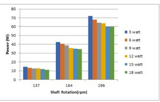
Figure 10. Graph of the relationship of electric power to shaft speed with variations in load on a modified 3 blade savonius wind turbine
