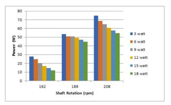
Figure 11. Graph of the relationship of electric power to shaft speed with variations in load on a conventional 3-blade Savonius wind turbine
