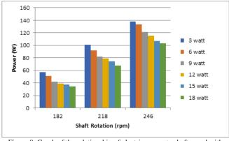
Figure 8. Graph of the relationship of electric power to shaft speed with variations in load on a modified 2-blade savonius wind turbine
