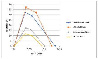
Figure 12. Graph of the relationship between efficiency and tordque with variations in wind turbine blades
