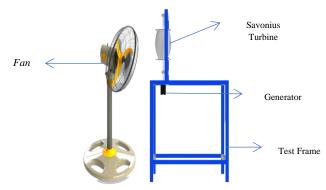
Figure 5. Testing image of savonius turbine with fan
