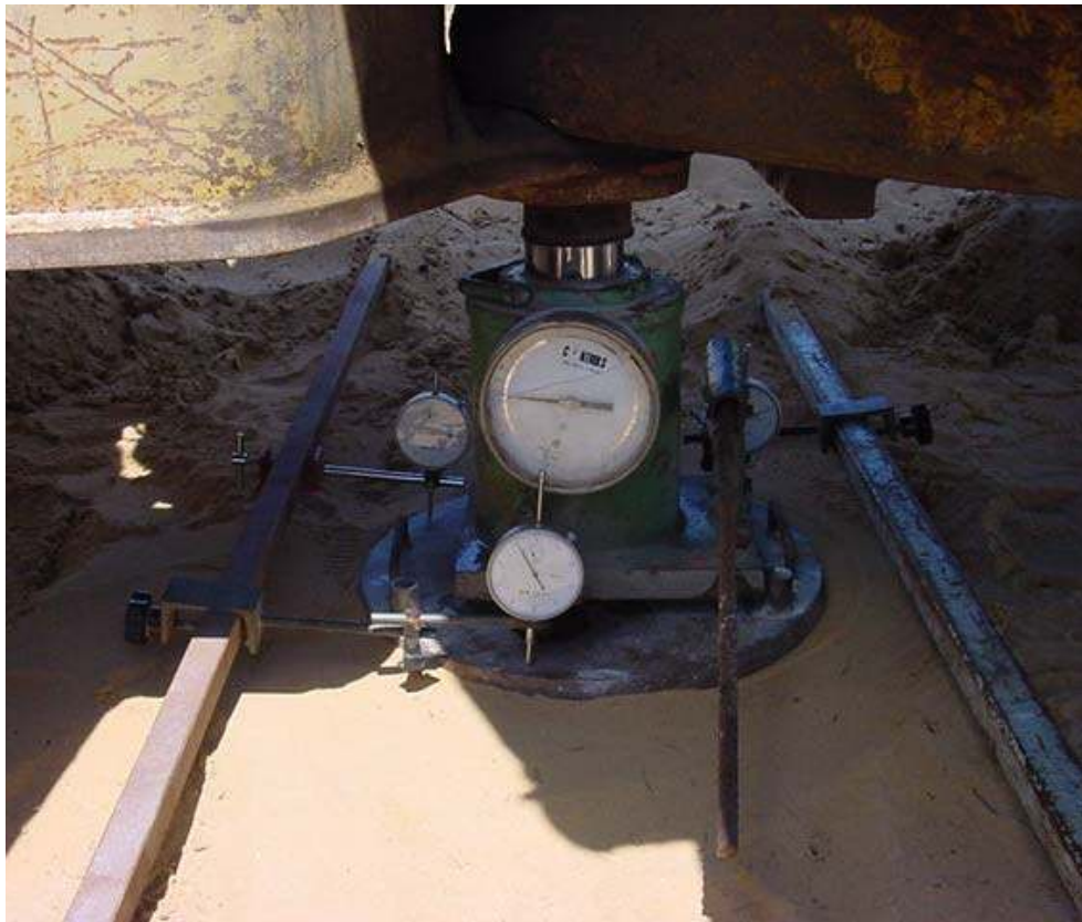
Figure (4.1): Arrangement for plate load test set-up
