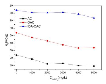
Figure 4. Effect of ion strength on the copper ion removal AC, OAC, and IDA-OAC.
