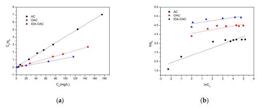
**Figure 6.** (a) Langmuir isotherm and (b) Freundlich isotherm model plots of AC, OAC, and IDA-OAC adsorption for Cu(II).
