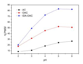
Figure 3. The impact of pH on the copper ion removal of AC, OAC, and IDA-OAC.
