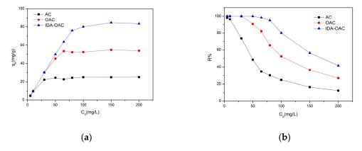
**Figure 5.** The adsorption capacity (**a**) and the removal efficiency (**b**) for AC, OAC, and IDA-OAC in the different initial concentrations.
