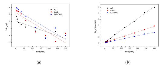
**Figure 8.** Linear plots of (**a**) pseudo-first-order kinetic and (**b**) pseudo-second-order kinetic models of AC, OAC, and IDA-OAC adsorption for Cu(II).
