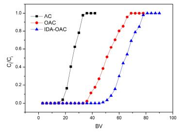
Figure 10. Column sorption of copper for AC, OAC, and IDA-OAC at initial concentration 50 mg/L.
