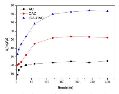
Figure 7. Effect of contact time for the adsorbents on the Cu(II) sorption.
