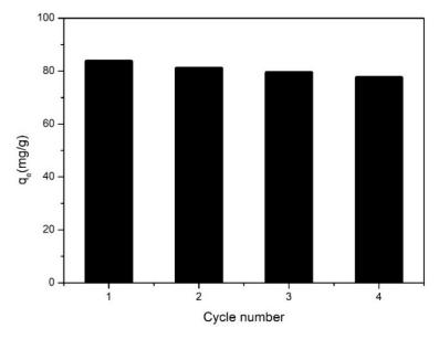
Figure 9. Variation in adsorption of Cu(II) in cycles of regeneration from IDA-OAC.
