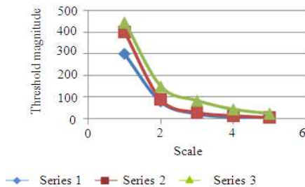
Fig. 2: Graph indicating relationship of the thresholded coefficients with the scale. Series 1, Series 2 and Series 3 are for standard deviations of 20, 30 and 50 respectively
