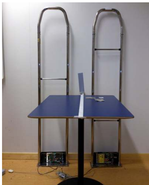
Figure 11. EAS detection gate setup where the gates have been turned side by side to test the reading range of EAS tags positioned in front of the gates.
