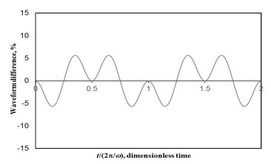
**Figure 9.** Difference between elliptic cosine and simple cosine (c/a = 0.5, k = 5,  $w/w_o = 3$ ,  $\xi = 0.02$ , single cavity, nonlinear solution).
