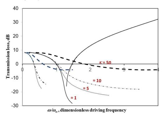
**Figure 4.** Transmission loss ratio versus excitation frequency for various excitation magnitudes  $(c/a = 0.5, \xi = 0.02, \text{ single cavity}).$
