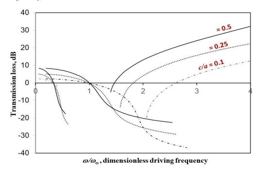
**Figure 6.** Transmission loss ratio versus excitation frequency for various cavity depths (k = 5,  $\xi = 0.02$ , single cavity).
