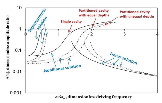
**Figure 7.** Amplitude ratio versus excitation frequency for various cavity cases (c/a = 0.5, k = 5,  $\xi = 0.02$ ).
