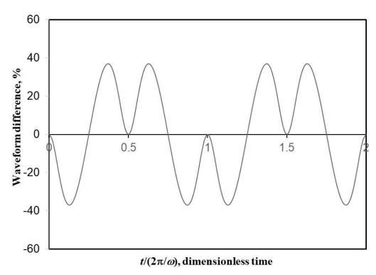
**Figure 11.** Difference between elliptic cosine and simple cosine (c/a = 0.5, k = 50,  $w/w_0 = 3$ ,  $\xi = 0.02$ , single cavity, nonlinear solution).
