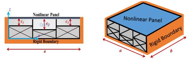
Figure 1. Nonlinear panel backed by a partitioned cavity.
