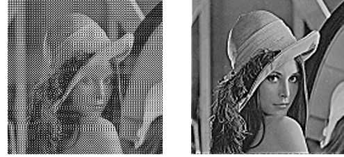
Figure 2 the experimental results of Lena 256x256 (a) Direct Inverting (Eq.3) PSNR only 6.5B (b) Laplacian filter (Eq. 4) + Bilinear, PNSR=19.8dB
