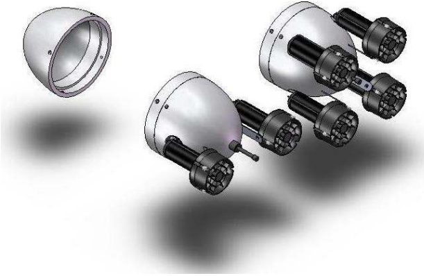
Fig. 3. Examples of end sections, showing a simple nose cone and different types of thruster assemblies. Note the dummy plug in the middle of the thrusters, used to charge the batteries (through and extension cable) once the vehicle is recovered.
