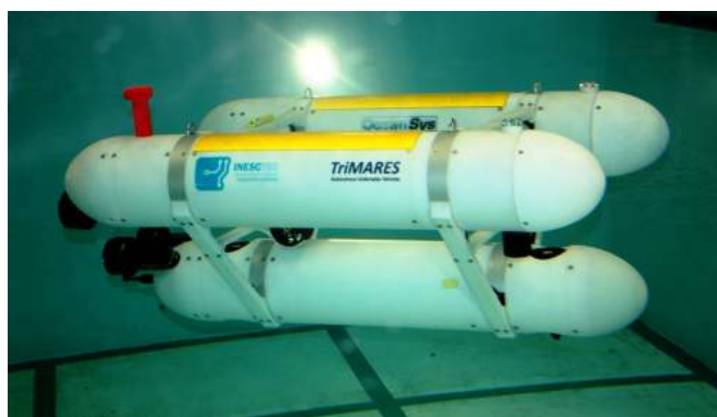
Fig. 9. The TriMARES hybrid AUV/ROV during water trials, June 2011.
