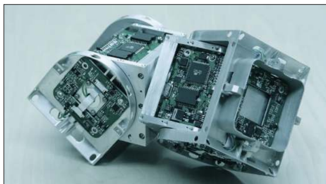
Figure 2. The Superbot modules have three rotational degrees of freedom and are designed to operate in real-world scenarios. Each Superbot module fits within a 168 \times 84 \times 84 \text{ mm}^3 rectangular box. (Picture courtesy of Polymorphic Robotics Laboratory, University of Southern California, Dr. Wei-Min Shen.)
