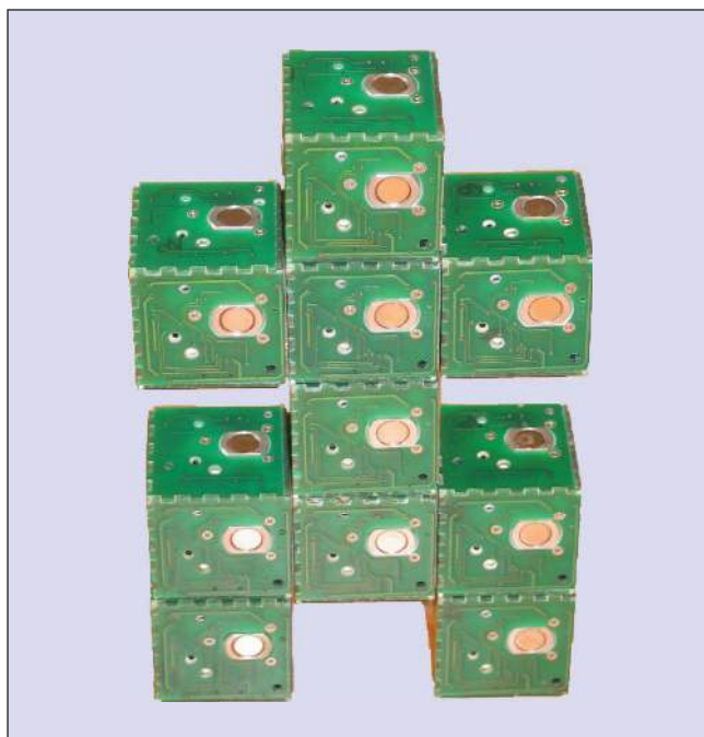
Figure 6. The Miche system consists of 45-cm cubic modules capable of forming 3-D structures. The modules contain batteries, two microprocessors, IR communication, and switchable permanent magnets for bonding with neighboring modules [51]. (Picture courtesy of Daniela Rus, Distributed Robotics Laboratory at MIT.)
