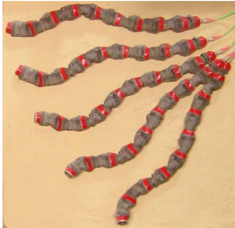
Movie S3. The snake robot performing differential turning in a sand bed due to an amplitude gradient in the horizontal wave.
