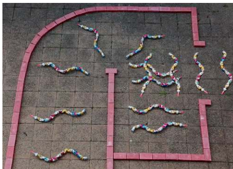
Movie S6. The snake robot (at 3\times speed) navigating a trackway using the three turn types described in this paper.
