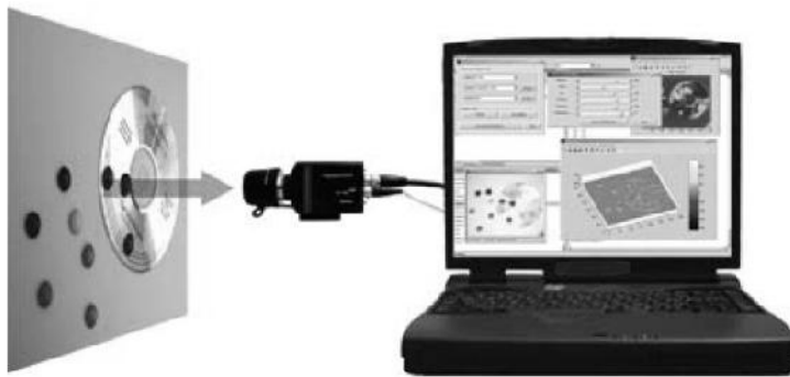
Figure 5: MATLAB interface with the scientific camera using Images Acquisition Toolbox
