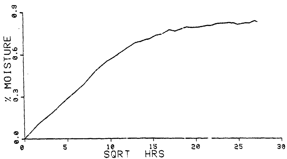
Figure 26. Typical Diffusivity Curve for S2 Glass/3501-6 from MPLDT RH = 98%, Temperature = 65.5°C (150°F), Thickness = 0.86 mm (0.034 in)
