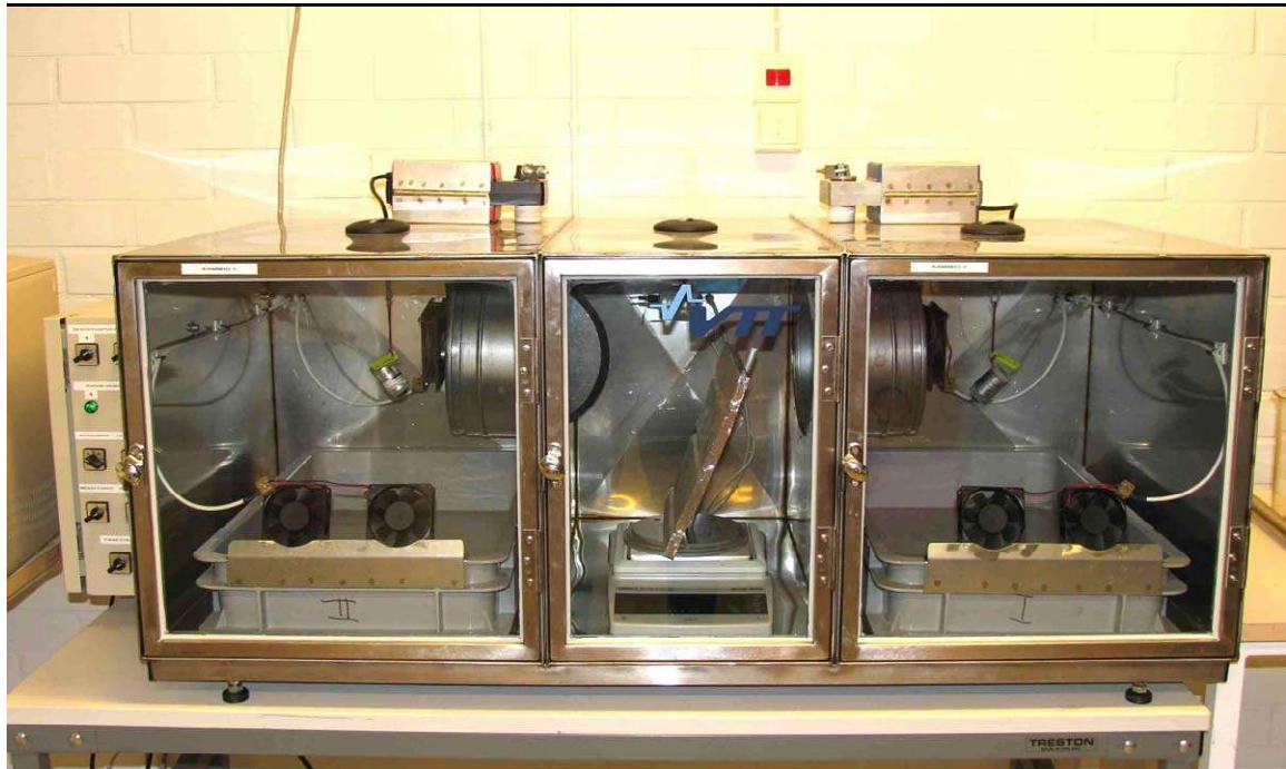
Figure 3-3: The experimental set-up at VTT. The sample is placed in the middle chamber and the low and high RHs are on each side.
