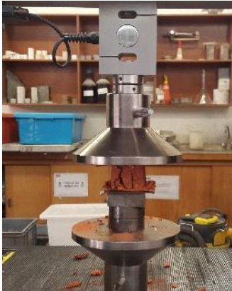
Fig 3. Mechanical tests setup: (a) brick compressive test; (b) epoxy and primer tensile test; (c) GFRP tensile test.
