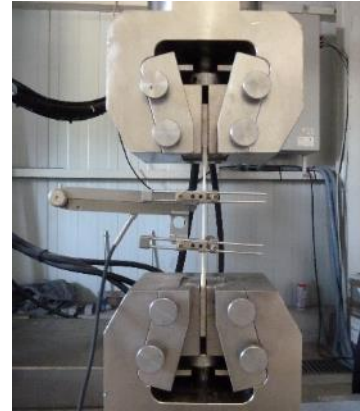
Fig 3. Mechanical tests setup: (a) brick compressive test; (b) epoxy and primer tensile test; (c) GFRP tensile test.
