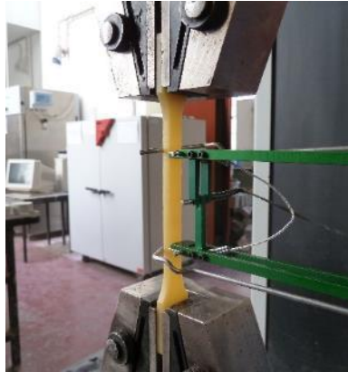
Fig 3. Mechanical tests setup: (a) brick compressive test; (b) epoxy and primer tensile test; (c) GFRP tensile test.
