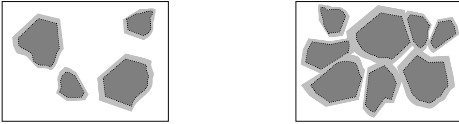
Figure 2. Illustration of a high water cement ratio to the left and a low water cement ratio to the right. Water, reaction products, CSH-gel, and cement grains are represented by the white area, lighter and darker shaded polygons respectively.
