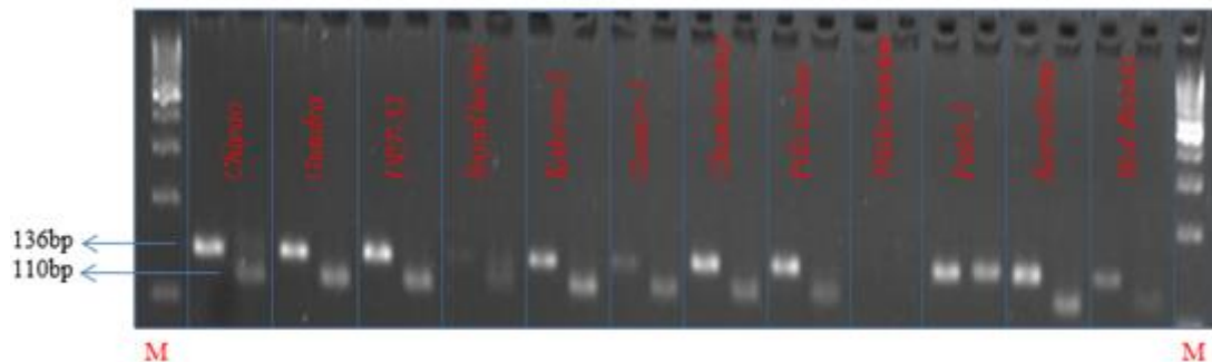
Fig 7. Amplification pattern of 12 selected rice varieties with SF28, a CAPS marker associated with grain length (GS3 gene) on 4% agarose gel. Two bands 110bp (marked with arrow) and 26bp (not visible above) are obtained after restriction digestion of the 136bp fragment by Pst I enzyme at 37°C for 1 hour. M: 100bp DNA ladder.
