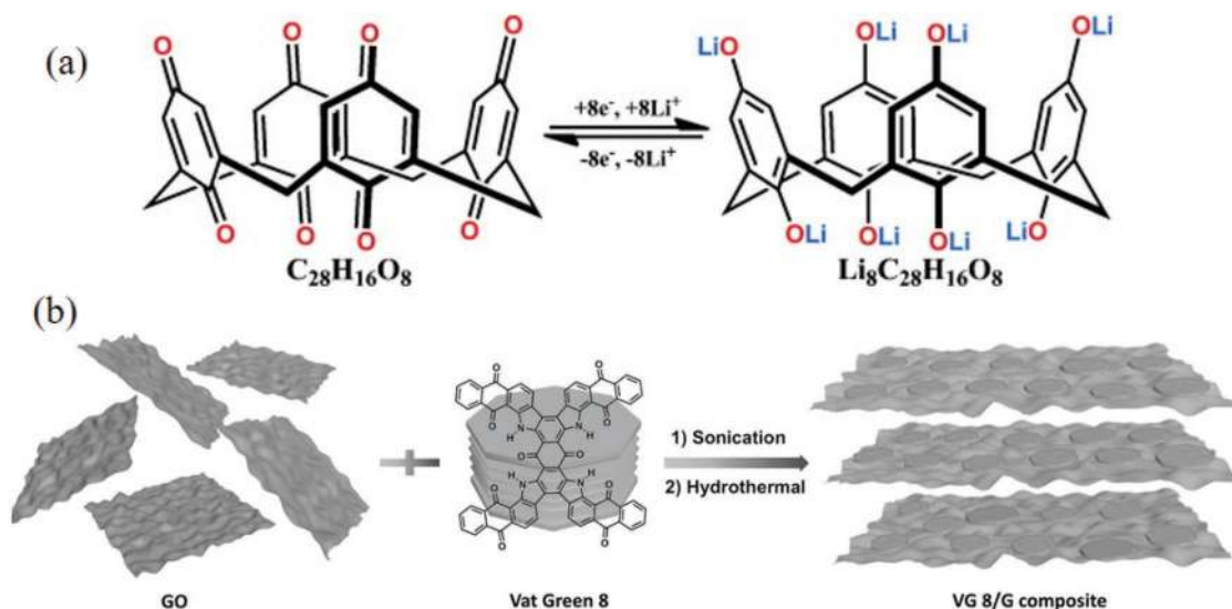
Figure 8. a) Molecular formula and proposed electrochemical redox reactions of C_{28}H_{16}O_8 ( C_4Q ) to give Li_8C_{28}H_{16}O_8 ; its C_{\text{theoretical}} is 446 \text{ mAh g}^{-1} . Reproduced with permission [145] Copyright 2013, Wiley-VCH. b) Schematic illustration of the synthesis of VG 8/G composite, which was formed through the disassembly of the Vat Green 8 crystal structure and subsequent reassembly on the graphene sheets. The main driving force for the formation of the VG 8/G hybrid architecture is the \pi - \pi interactions between Vat Green 8 and the graphene sheets. Reproduced with permission [146] Copyright 2016, Wiley-VCH.
