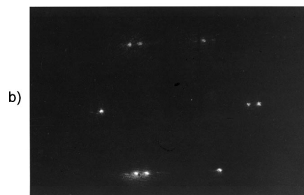
FIG. 2. Low energy electron diffraction (LEED) patterns of cleaned stepped Pt surfaces: (a) Pt(335) or Pt(S)-[4(111)×(001)], 145 eV; (b) Pt(779) or Pt(S)-[8(111)×(001)], 145 eV.
