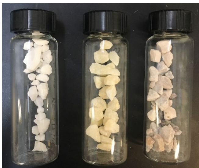
Figure 1. Three colored phases (white, yellow, and gray from left to right) of AC. Slow solidification and cooling at Dead Sea Magnesium (DSM) may have resulted in phase separation. Yellow is the primary phase in AC in terms of quantity.
