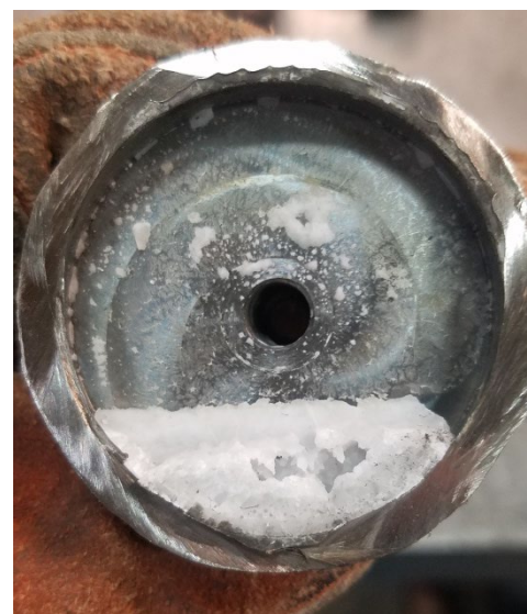
Figure 39. Trapped salt in the 20- \mu\text{m} filter casing
