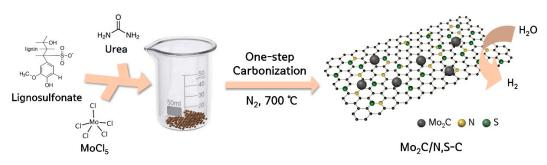
Scheme 1. Schematic illustration for the preparation of Mo<sub>2</sub>C/N,S-C.
