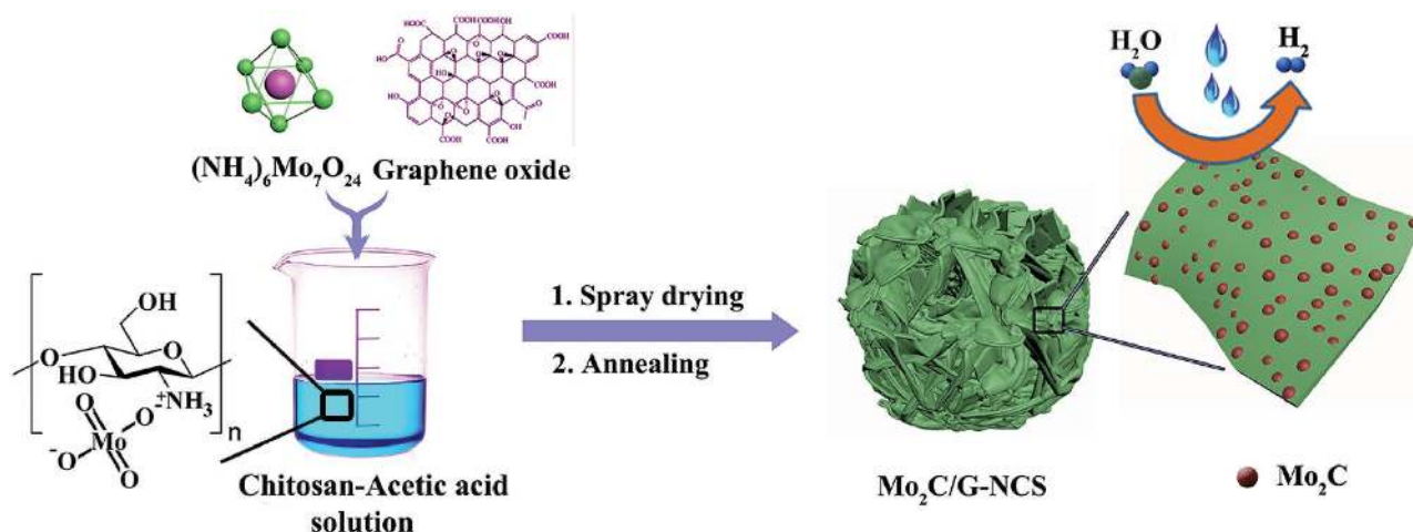
Scheme 1. Schematic illustration of the procedure for preparing Mo 2 C/G-NCS.
