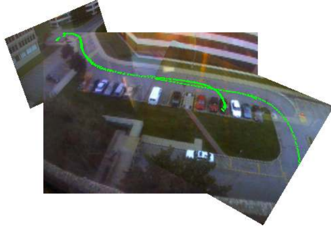
Figure 7: An example of an error. Two vehicles travelling close together (about two cars lengths apart) were assigned the same unique identifier.
