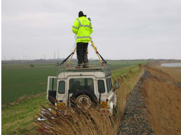
Figure 2 Laser scanning from vehicle roof – mobile set-up
