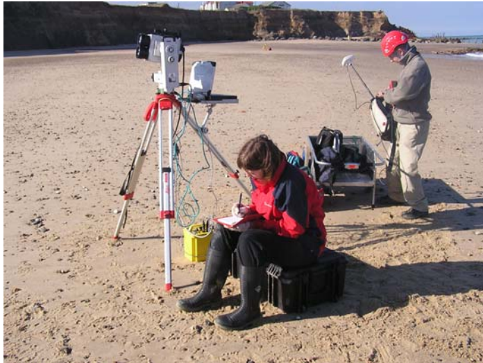
Figure 1 Laser scanner mounted on tripod – mobile set-up
