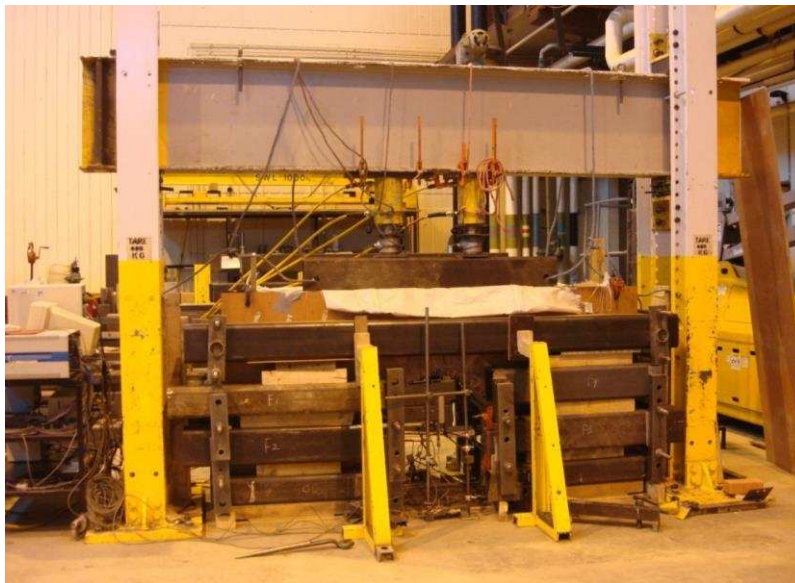
Fig 2. Loading system installation for uniform load (Chen, 2014)
