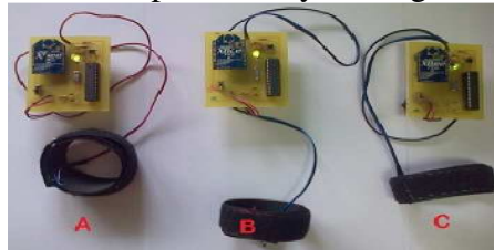
Fig. 5. Temperature and Heartbeat Monitoring Device using Zigbee
