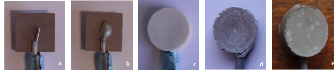
Figure 6. SMAG transducer manufacturing steps.
